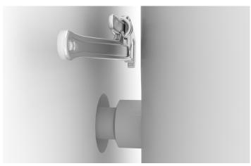
8. Fasten the basin to the brackets through the installation access openings with the provided fasters.
