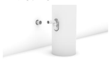
6. Rotate the basin so the back is facing towards the finish wall. Lift the basin and then lower it down into position using your outline (from step 1.) as a reference.
